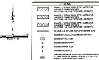
CONTRACTOR SHALL SAWCUT THE PERINETER OF THE REPAIR LIMITS AS SHOWN ON PLANS, REMOVE THE CONCRETE SLAB AND DAMAGED BASE IF NEEDED. DRILL HOLES FOR LONGITUDINAL AND TRAVERSE THE BARS OR DOWN BARS, PROVIDE LONGITUDINAL AND TRAVERSE STEEL CONTINUITY. PLACE AN NEEDED, DRILL HOLES FOR LONGITUDINAL AND TRAVERSE TIE BARS OR DOWEL BARS, PROVIDE LONGITUDINAL AND TRAVERSE STEEL CONTINUITY, PLACE AND FINISH CONCRETE AND RESTORE EXISTING JOINTS.
